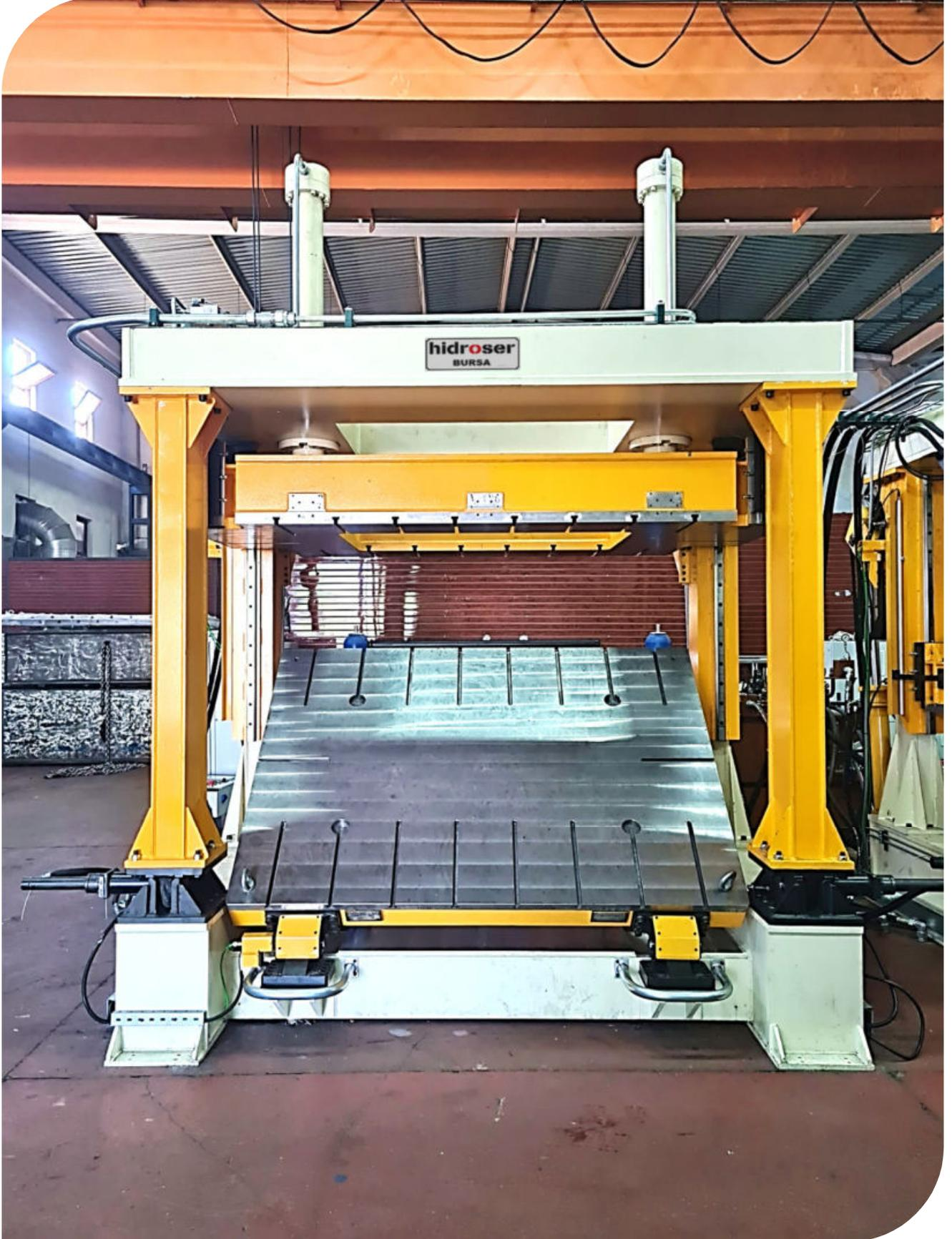
**10 TON HYDRAULIC PRE-HEATING DECK OVEN PRESS**
